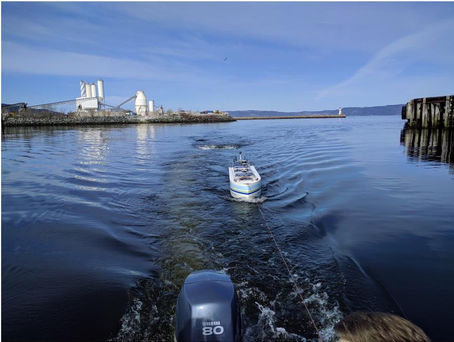
**Figure C.1:** Transport stage with drogue connected to ReVolt's aft.
