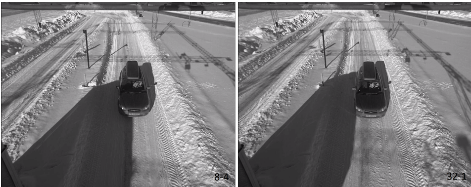
Figure 4.7: Reference image for sensor configuration test. Left: 8 accumulations and 4 oversampling. Right: 32 accumulations and 1 oversampling.
