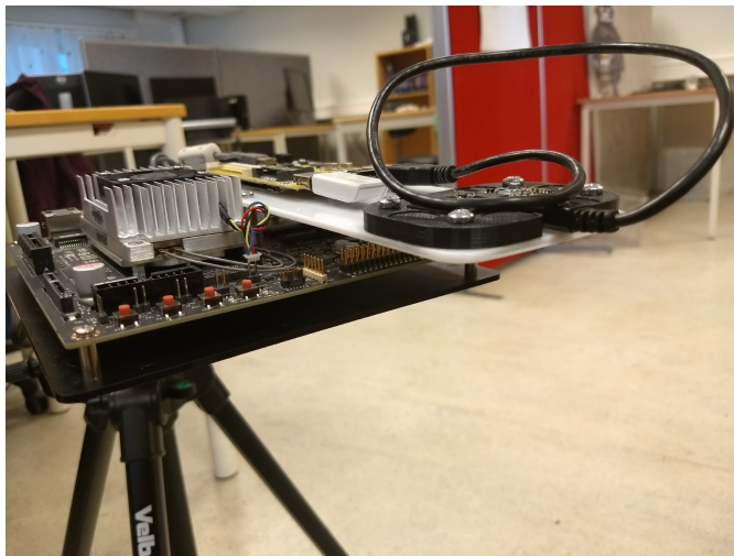
Figure 4.8: The complete system setup, stereo camera pointing downwards
