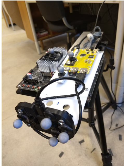
Figure 4.10: Retroreflective markers attached to the TX1
