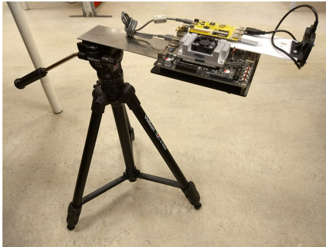
Figure 4.7: The complete system setup, stereo camera pointing outwards
