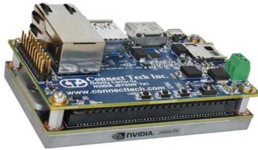
Figure 10.1: The Orbitty Carrier board mounted on a Jetson TX1 module
