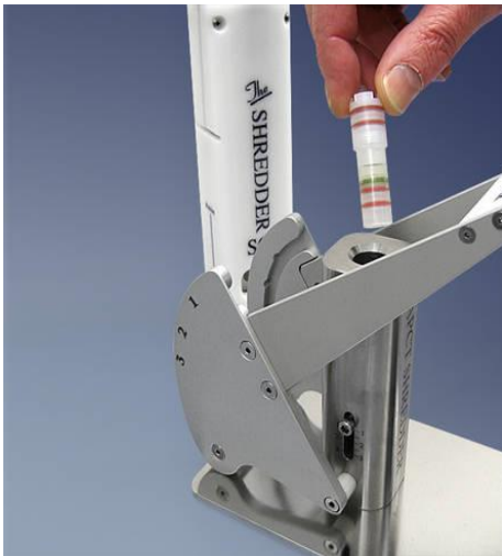
Figure 4.3: The correct positioning of the shredder tube into the shredder base with the ram side of shredder tube facing downwards
