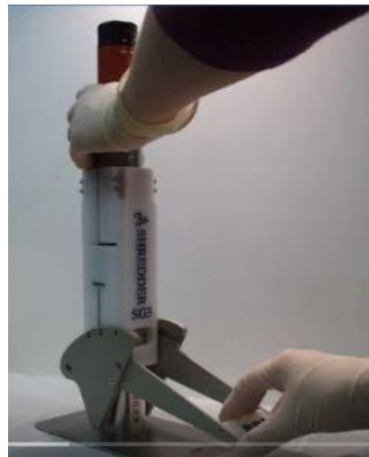
Figure 4.4: Pressing down of the driver and adjusting the lever into the suitable position
