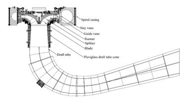
Figure 1. 2D view of the turbine model. Retrieved from [11].
