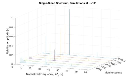
Figure 4.22: Frequency spectrum for simulations at  $\alpha = 14^{\circ}$  at different monitor points.
