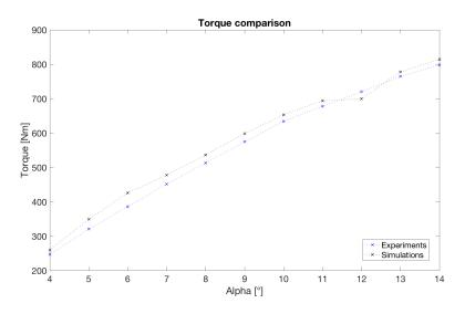
Figure 4.1: Comparison of torque between experiments and numerical results.
