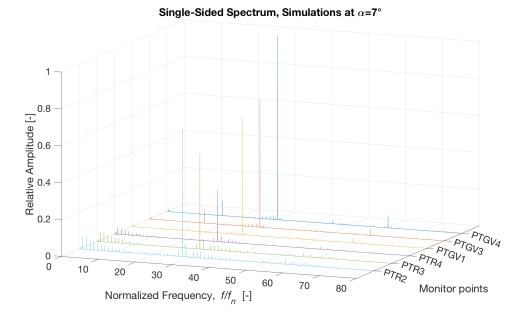
Figure 4.18: Frequency spectrum for simulations at  $\alpha = 7^{\circ}$  at different monitor points.
