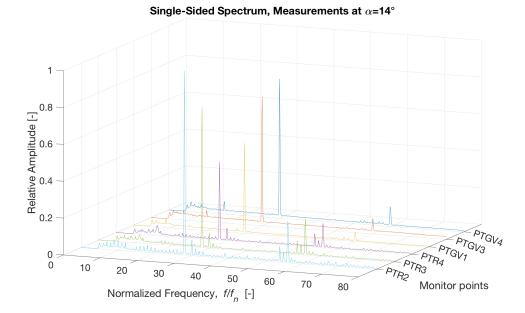
Figure 4.23: Frequency spectrum for measurements at  $\alpha = 14^{\circ}$  at different monitor points.
