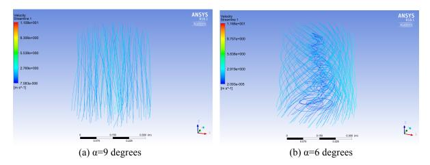
**Figure 7.** Velocity streamlines for  $\alpha$ =9 degrees (a) and  $\alpha$ =6 degrees (b) from the outlet of the runner to the outlet of the draft tube part. It is clear from the streamlines that there is a significant swirl component when the turbine is operating off-design.
