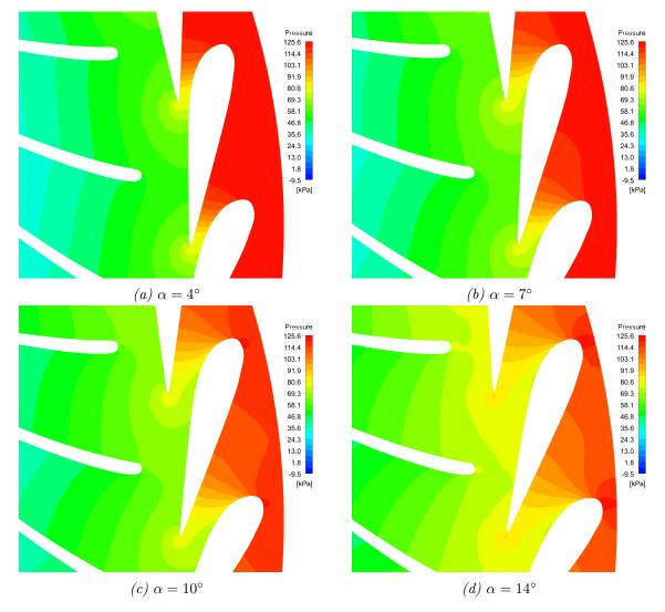
Figure 4.7: Pressure contour for four different alphas in a rotating frame of reference.
