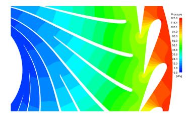
Figure 4.6: Pressure contour for  $\alpha = 10^{\circ}$  in a rotating frame of reference.
