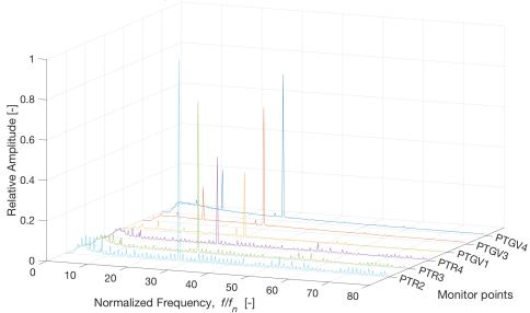
Single-Sided Spectrum, Measurements at  $\alpha {=} {\rm 4^\circ}$
