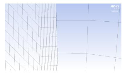
Figure 4.15: The interface between the mesh in the guide vanes (left side) and the mesh in the runner (right side).
