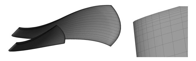
**Figure 4.** To the left is the mesh for the main blade and the splitter blade. To the right is a close-up of the leading edge of the main blade. The mesh is refined close to edges.
