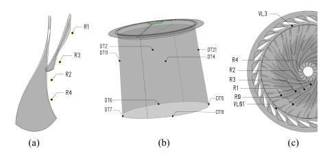
Figure 3. Monitor points and their location in one runner passage (a), draft tube (b) and vaneless gap (c).
