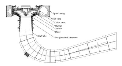
Figure 2.1: 2D view of the turbine model. Retrieved from [16]
