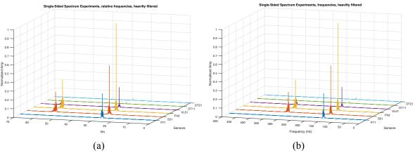
Figure 2. The spectrum for all sensors. Frequency f is relative to  $f_n$ . Amplitude in kPa.
