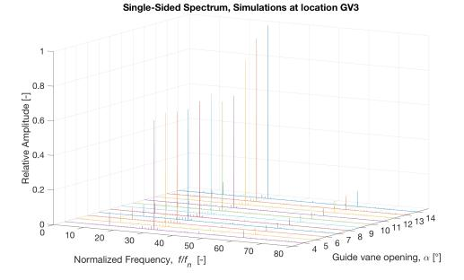
Figure 4.13: Frequency spectrum for monitor point PTGV3 at different alphas.
