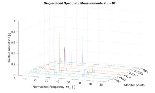
Figure 4.21: Frequency spectrum for measurements at  $\alpha = 10^{\circ}$  at different monitor points.
