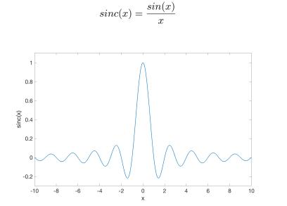
Figure 3.7: Representation of the sinc(x) function and the resulting side lobes.
