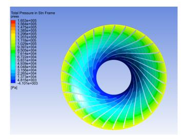
Figure 6. Contour of total pressure in a stationary frame in the runner for steady state simulation at  $\alpha$ =9 degrees.
