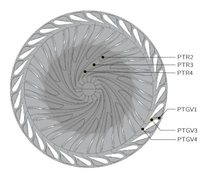
Figure 3.6: An overview of the location of the monitor points used for simulations and analysis.
