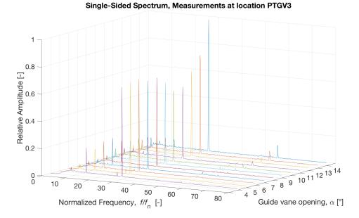
Figure 4.14: Frequency spectrum for experimental measurements at sensor PTGV3 at different alphas.
