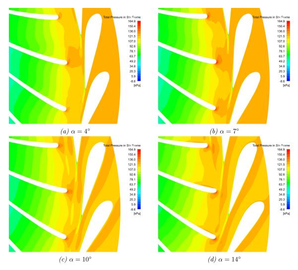
Figure 4.5: Pressure contour for four different alphas in a statinary frame of reference.
