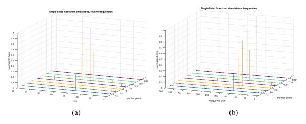
Figure 8. Frequency spectrum obtained through CFD for BEP. Frequencies are relative to  $f_n$  in a, while b shows the actual frequencies. Amplitudes are normalized against the highest peak.
