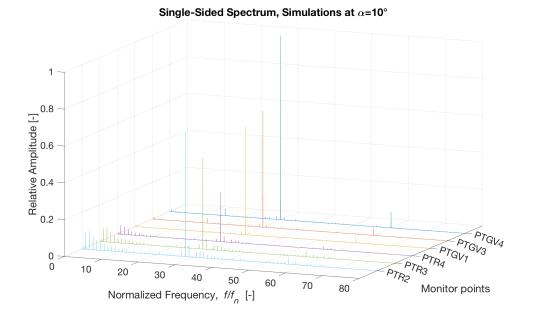
Figure 4.20: Frequency spectrum for simulations at  $\alpha = 10^{\circ}$  at different monitor points.
