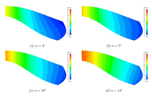
Figure 4.8: Pressure contour for the pressure side of a single main blade.
