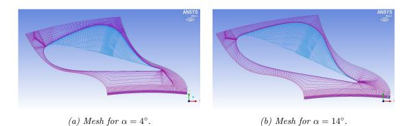
Figure 3.3: Comparison of meshes for two different alphas.
