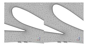
Figure 3.2: Figure shows the final guide vane position during part load (left) and high load (right) when using mesh deformation. Retrieved from [24].
