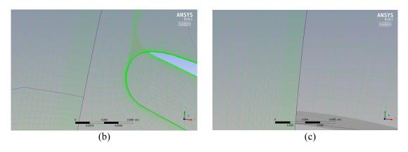
Figure 5. Figure (a) shows the modified mesh for the guide vanes at  $\alpha$ =9 degrees together with the runner. It can be seen from figure (b) that there is a large difference in cell size from guide vane to runner. This becomes even more evident in the runner passages as seen in figure (c).
