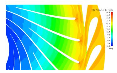
Figure 4.4: Pressure contour for  $\alpha=10^\circ$  in a stationary frame of reference.
