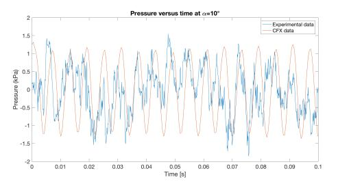
Figure 4.10: Pressure versus time for experiments and simulations. The pressure curve for the experiments has been shifted. Because of the outlet condition, the pressure in the simulations are wrongly predicted, but change in pressure is correct.
