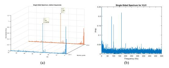
Figure 9. The frequencies observed in the draft tube is shown in figure a . Figure b shows the unfiltered frequency spectrum for sensor VL01.
