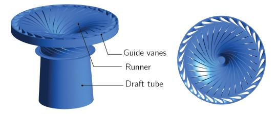
Figure 3.1: An overview of the modelled flow passage.
