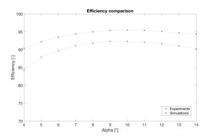
Figure 4.2: Comparison of efficiency between experiments and numerical results.
