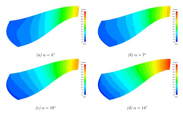
Figure 4.9: Pressure contour for the suction side of a single main blade.
