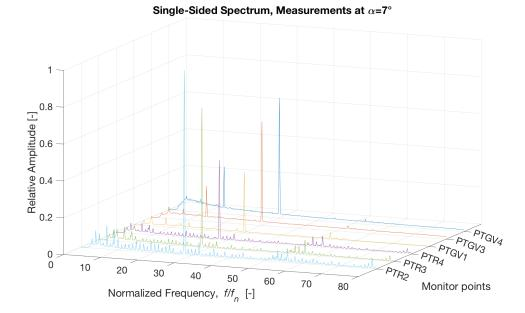
Figure 4.19: Frequency spectrum for measurements at  $\alpha = 7^{\circ}$  at different monitor points.
