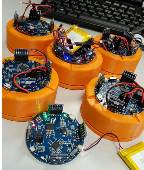
Figure 4.12: Six real-world swarm robot devices.
