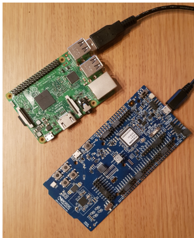
Figure 4.13: The Thread Border Router / MQTT-SN gateway solution.
