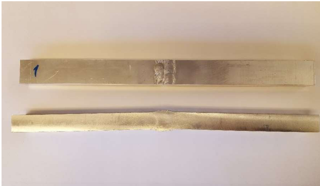
FIGURE 31: WELDED JOINT 20 MM THICK
