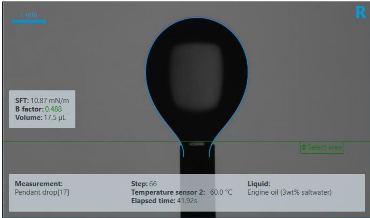
Figure 23: Measuring the IFT between engine oil and synthetic brine at 60 °C
