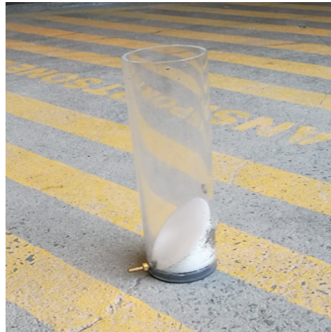
Figure C.1: The figure shows the cutting separator with the cutting outlet on the bottom left. The floor is tilted 45^\circ , guiding the cuttings towards the outlet.
