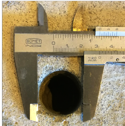
Figure 9.31: Measured OD of a hole drilled in granite with the NTNU bit.
