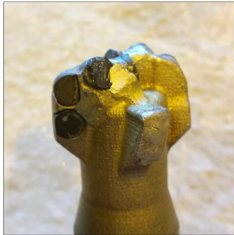
Figure 9.30: Chipped cutters on the NTNU bit. Cutters at the gauge are less damaged than those close to the center.
