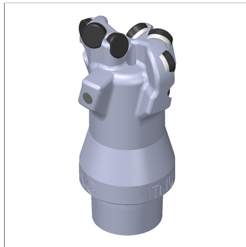
Figure 6.34: Final custom bit 3D model, including cutters, metal inserts, coating and logos.
