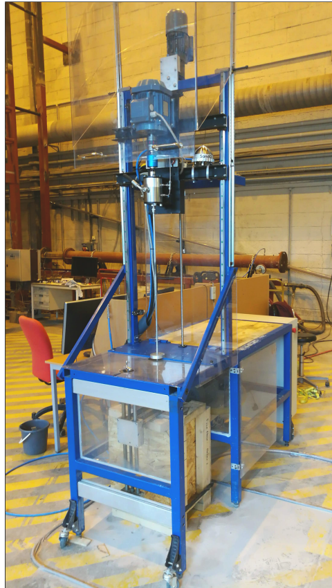
Figure 6.10: Photography of final rig entered for the Drillbotics competition.
