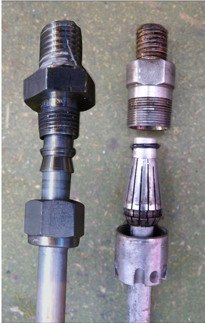
Figure 6.40: Old and new BHA tooljoint.
