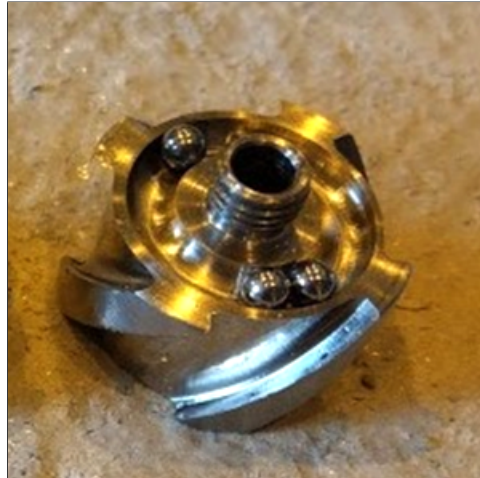
Figure 6.42: Freely moving balls in the dynamic stabilizer.
