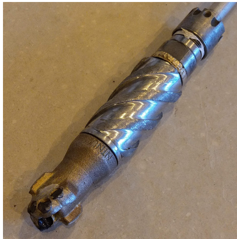
Figure 10.3: The final BHA configuration used in the competition run, featuring the NTNU bit, stabilizer housing DH sensors and pipe connection.
