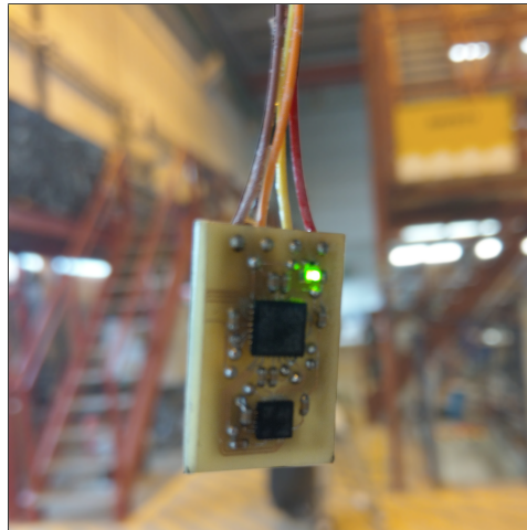
Figure 6.39: Downhole sensor card with accelerometer, gyroscope and thermometer.
