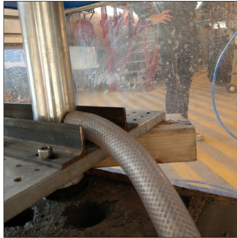
Figure 6.13: Semi-closed loop system with neoprene layer sealing the interface between rock formations and the riser guide. The water is guided through the rubber hose directly to the drain.
