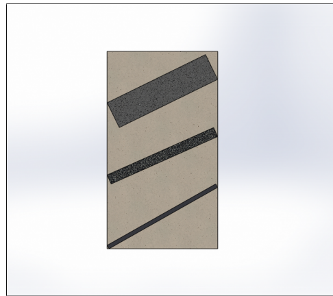
(d) Mixed1. Made with three inclined layers of tile (1.2 cm), basalt (2.5 cm) and shale (7 cm). The inclination angle is between 23^\circ and 28^\circ .
