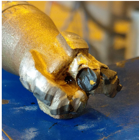
Figure 10.4: Showing the NTNU bit in its condition after drilling through the competition rock. Significant damage is evident on all but the gauge cutters.
