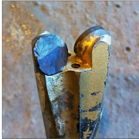
Figure 9.29: Chipped cutter on the DSATS bit.
