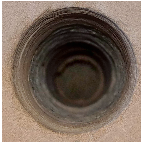
Figure 10.18: Showing the competition borehole, ready for completions. The boundary between sandstone and pebbled cement can be seen a few centimeters down. A smooth surface was obtained, with some imperfections noticeable especially in formation transitions. The hole was drilled through the entire competition rock, and the very last layer is actually the outline of the wooden crate's floor.
