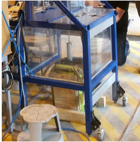
Figure 10.2: Showing the formation located underneath the miniature rig on the competition day. Two straps are used to secure the formation, connecting to four floor-mounted hooks.
