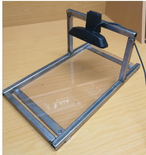
Figure C.2: The figure shows the setup of the screen and the camera for picture analysis of the cuttings in the return flow.
