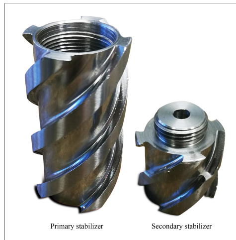
Figure 6.41: Photography of the primary and secondary stabilizer subs of the new BHA.
