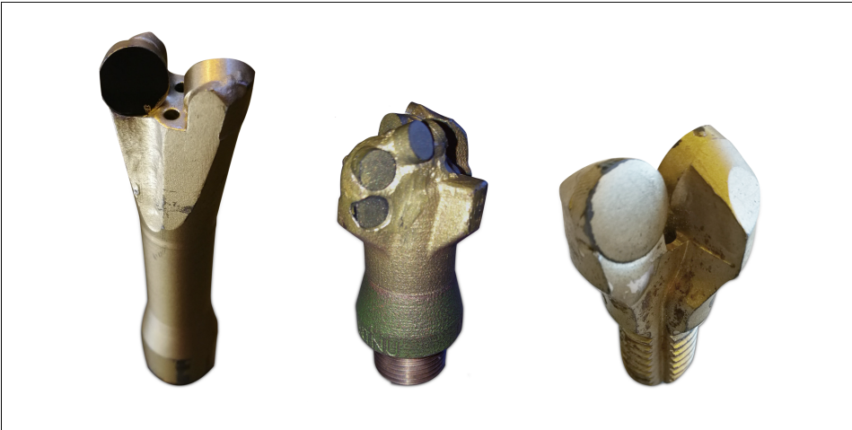
Figure 9.22: Drill bits involved in performance testing. From left to right: DSATS, NTNU and Alibaba bit. The bits are not to scale.
