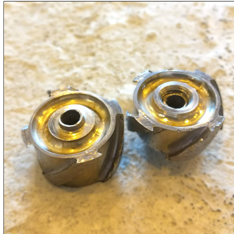
Figure 9.21: Broken pin with threads on the dynamic stabilizer subs. The broken male part is stuck inside the corresponding female part.
