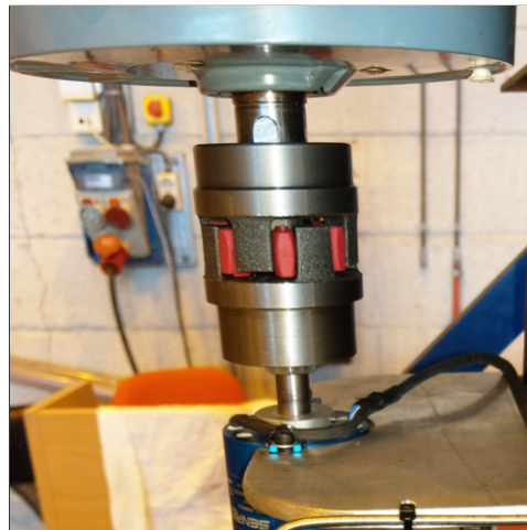
Figure 6.8: Universal coupling mounted below the top drive motor.
