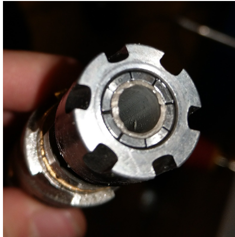
Figure 9.4: Twist-off occurred mainly at the bottom connection, always in the transition from pipe to connection.
