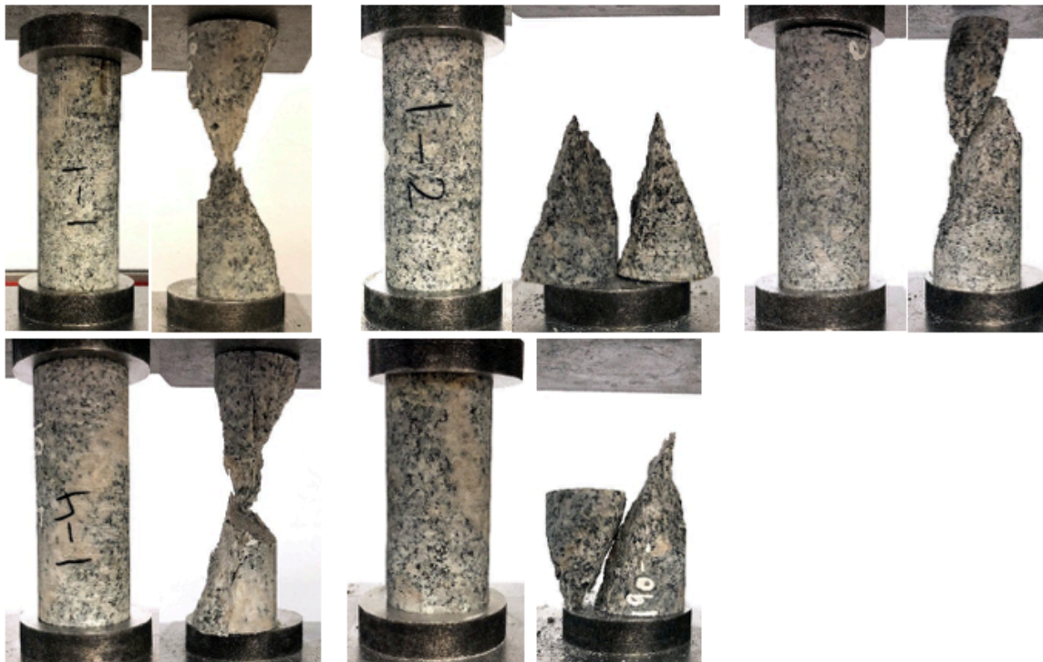
Figure 40: Modes of failure of the test specimens (Photo: N. Haugen)
