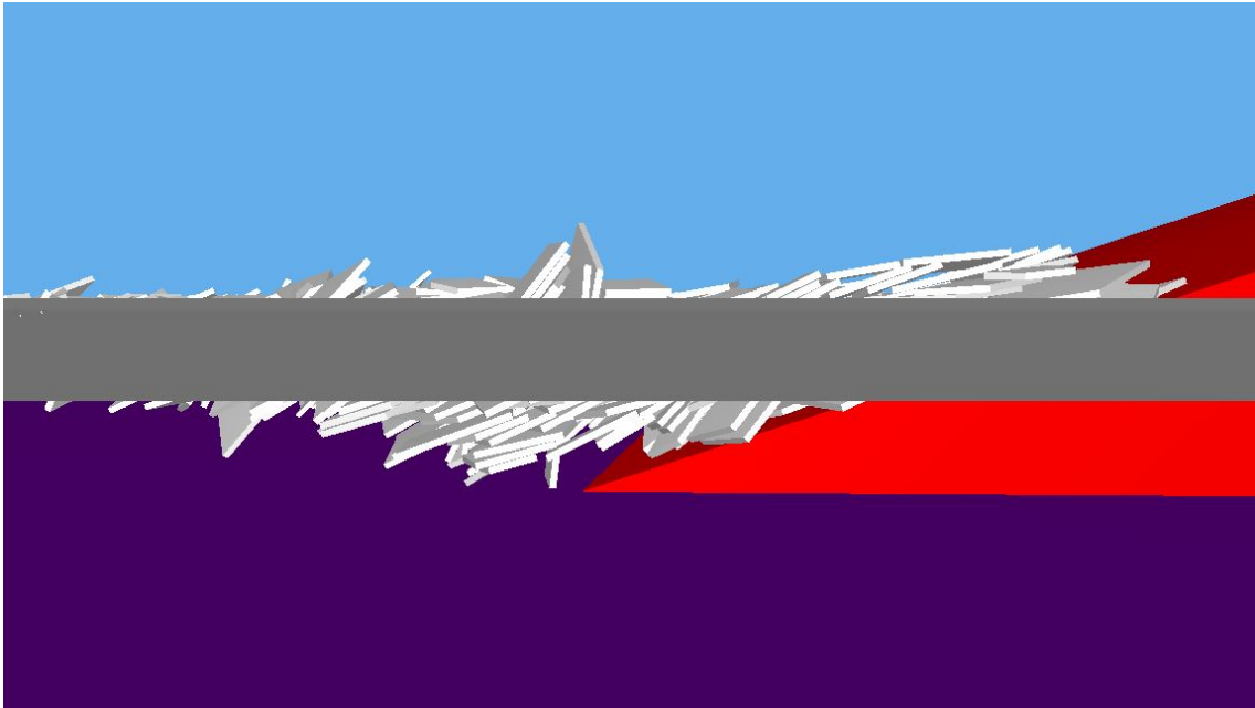
Figure 5-12 Pile-up: Stage 3 - Rubble pile development
