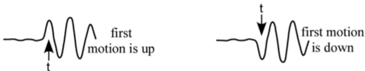
Figure 3.16: First motion of an earthquake is either up (left) or down (right) (Cronin, 2010).
