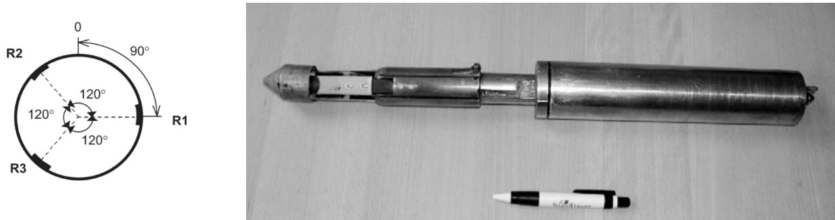
Figure 3.7: Strain gauge rosette configuration and a photo of the Borre probe. Modified after Sjöberg et al. (2003).
