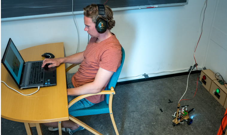
Figure 4.1: Experimental setup. The computer (left), is used to control the ROV into holes in wooden box (right).
