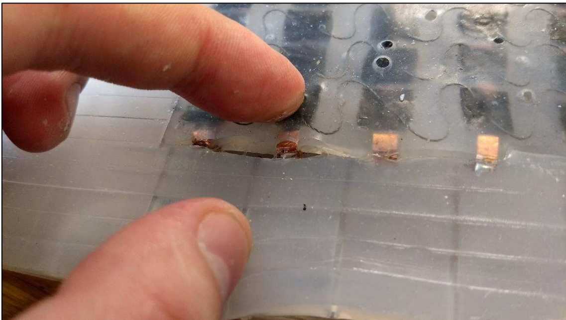
Figure 4.20 - Gap between sensor skin and foil body where silicone didn't cure
