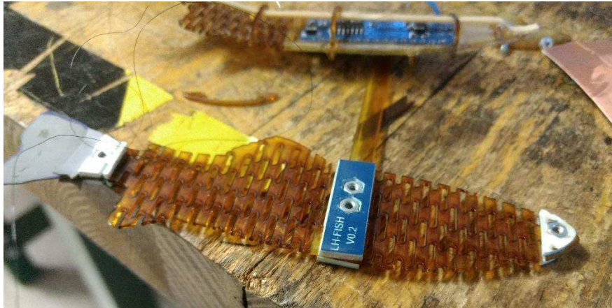
Figure 4.11 - Fish inner body glued together
