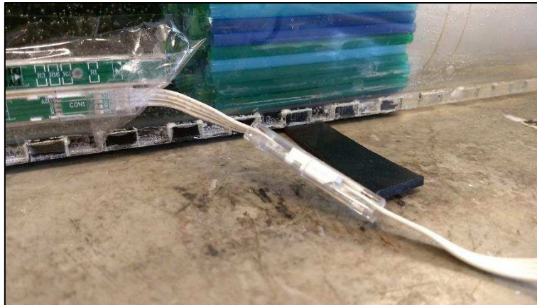
Figure 2.2 - Rubber strip under tank
