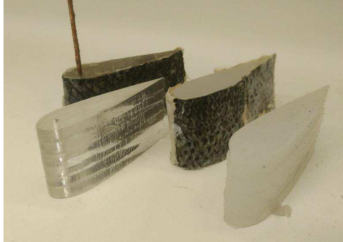
Figure 3.3 - The four different surface effect samples.
