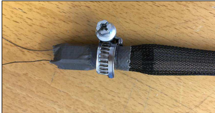
Figure 6.1 - McKibben muscle with CFRSS sensor installed
