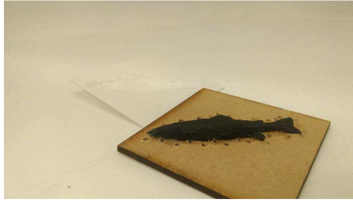
Figure 3.11 - 3D-printed and vacuum formed mould for silicone casting
