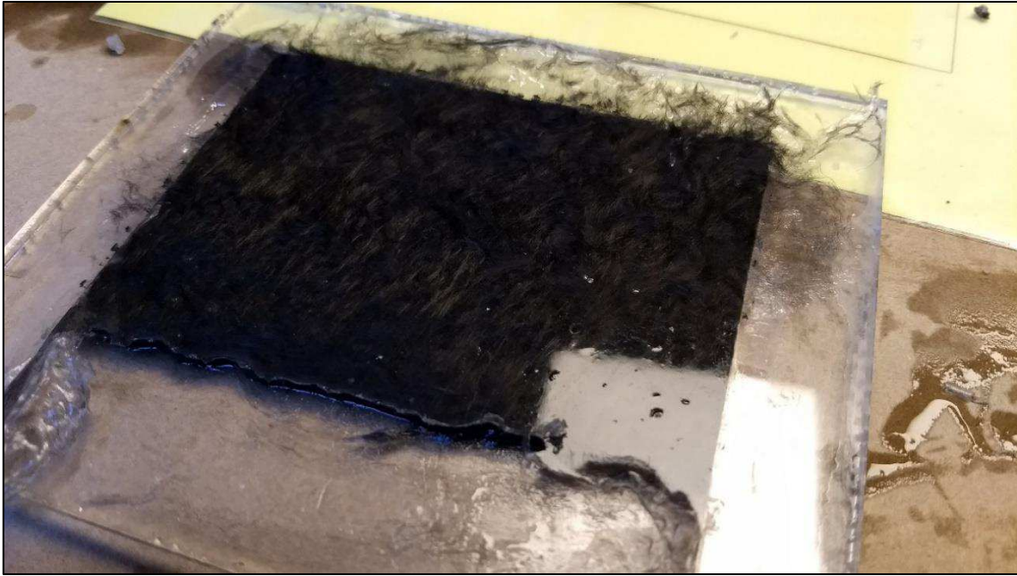
Figure 4.24 - Sensor sheet during casting
