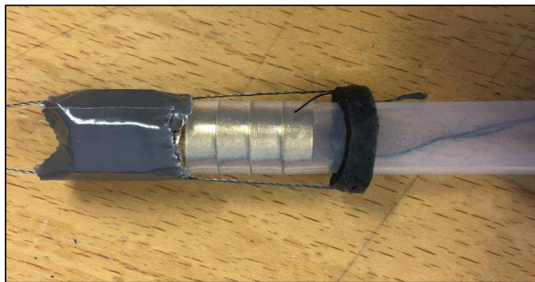
Figure 6.2 - Sensor inside McKibben muscle
