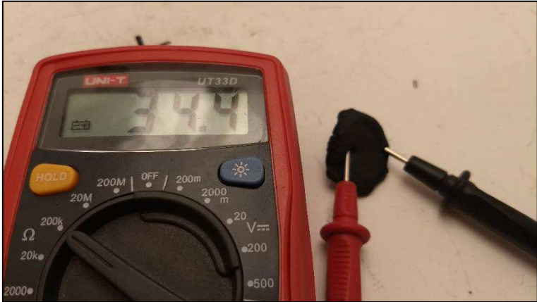
Figure 3.14 - Graphite infused clay before stretching.
