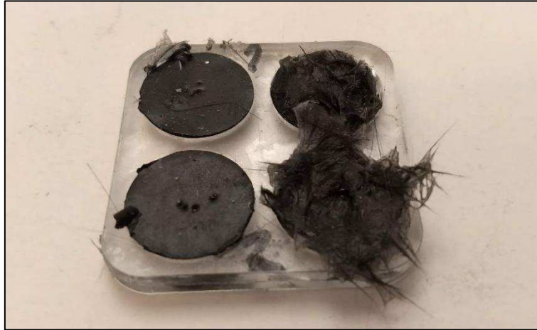
Figure 3.17 - Silicone samples . Samples mixed with graphite to the left and carbon fibers on the right.
