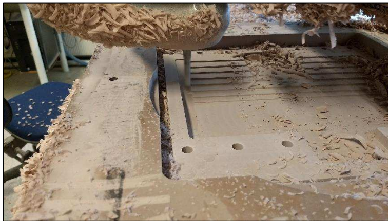
Figure 4.29 - Mold being cut
