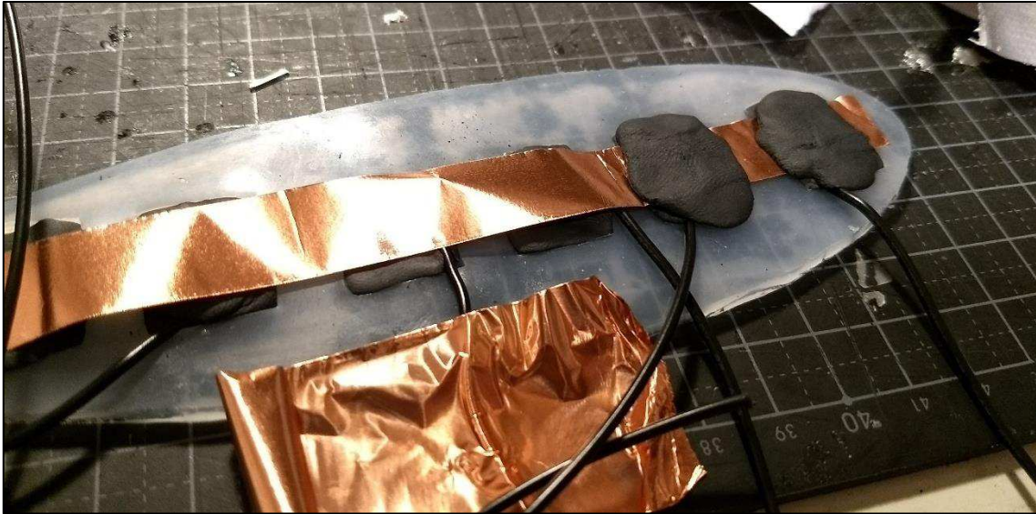
Figure 3.16 - Play dough sensors being placed into silicone foil
