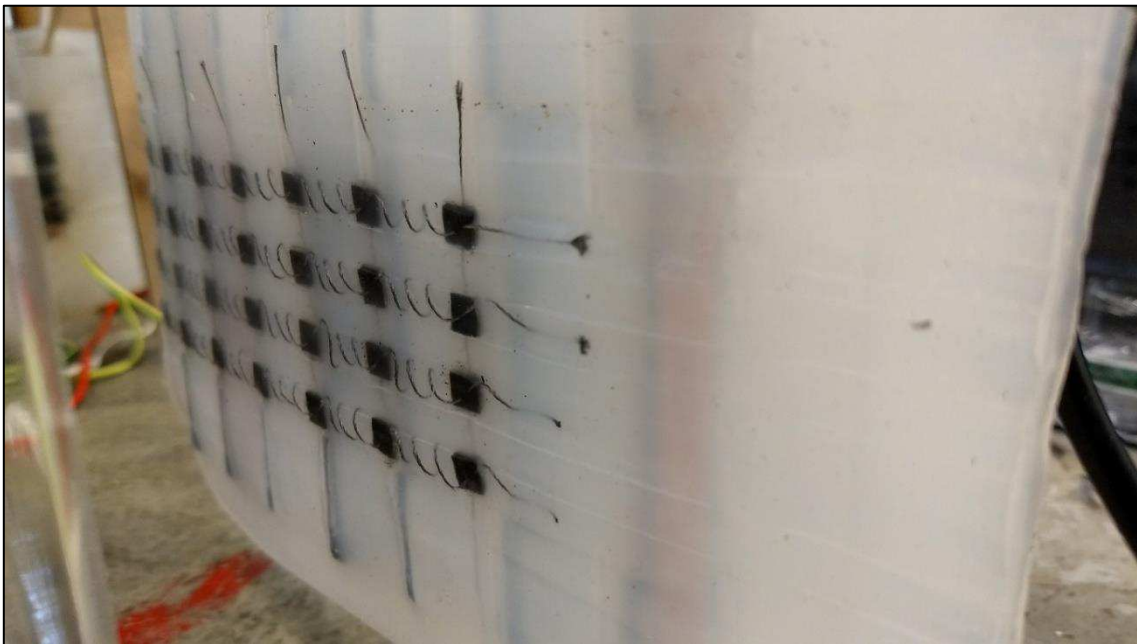
Figure 4.33 - Finished casting of hydrofoil with imbedded sensors
