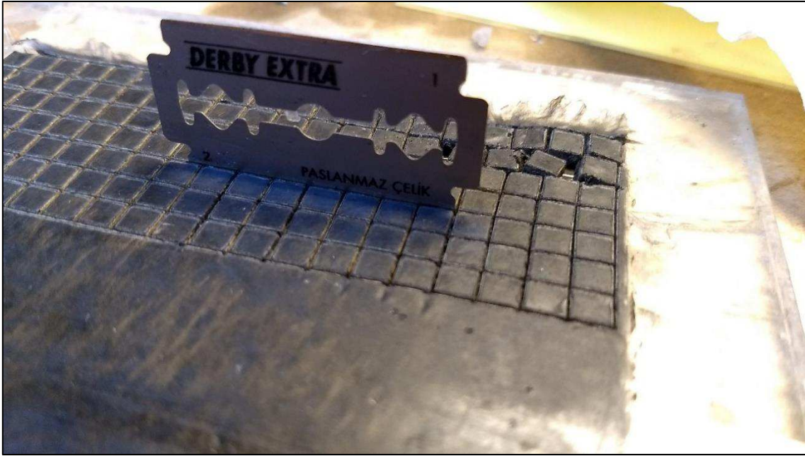
Figure 4.25 - Cutting sensors by following the laser cut path
