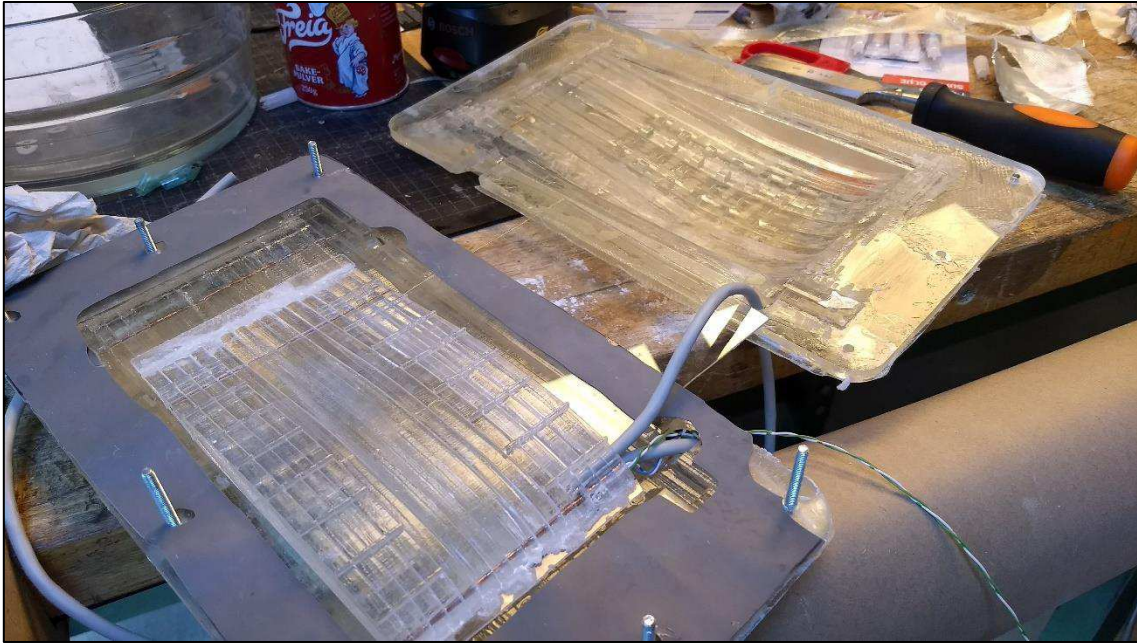
Figure 4.22 - Mold, inner core, gasket and locking screws before assembly and casting.
