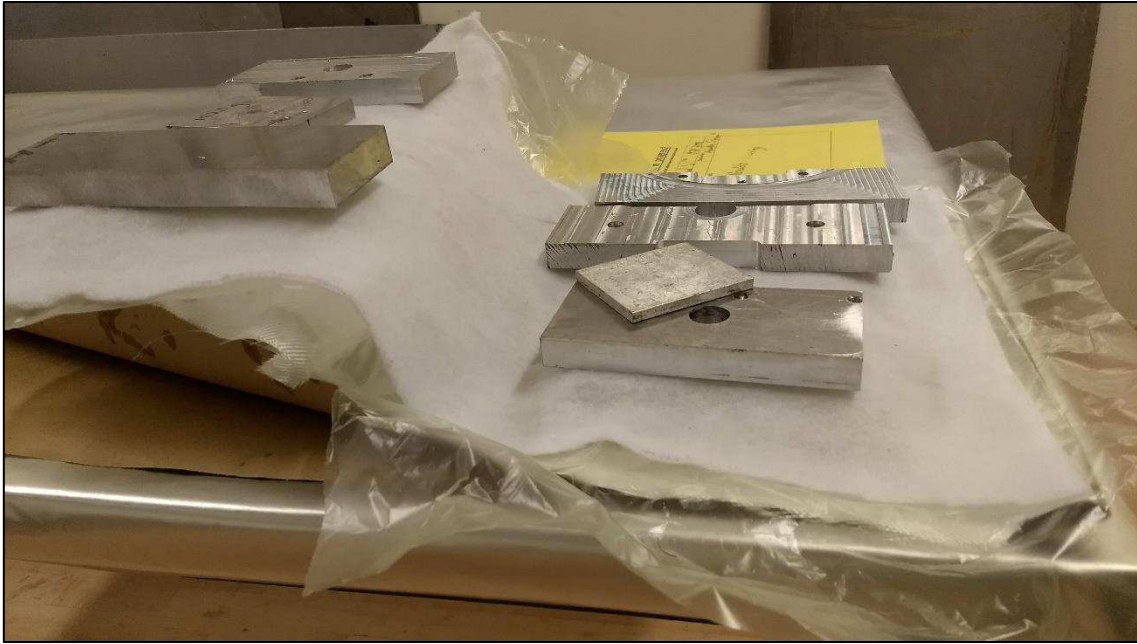
Figure 4.21 - Casting outer glass fiber-epoxy shell to mold. Fiber is covered with release film and breather material before weights were added.
