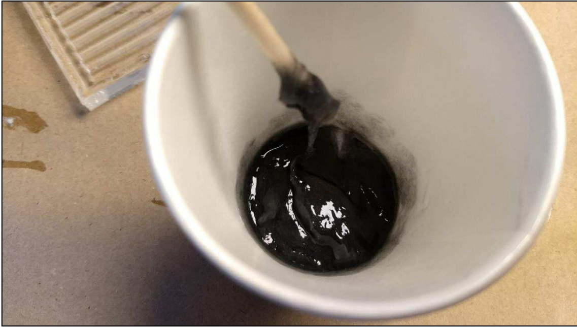
Figure 4.23 - Consistency pre-casting of the failed sensor silicone-fiber mix
