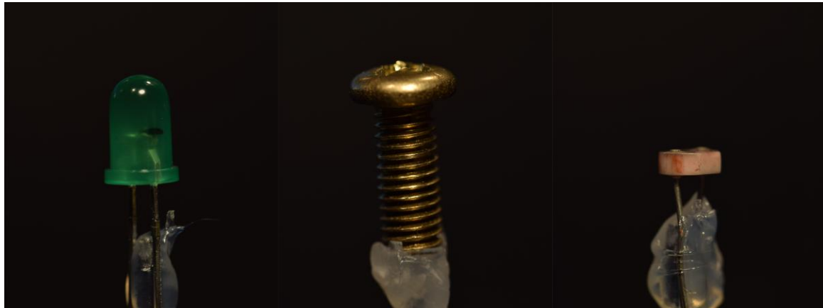
Figure 31: Typical objects that are difficult to scan with photogrammetry: LED, metal screw and photoresistor.
