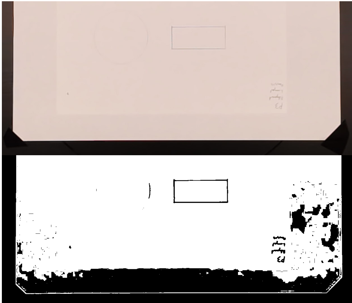
Figure 11: Captured BMP image of a test sample and the resulting binary PNM image after using the threshold function. Note the barely visible circle on the top image.
