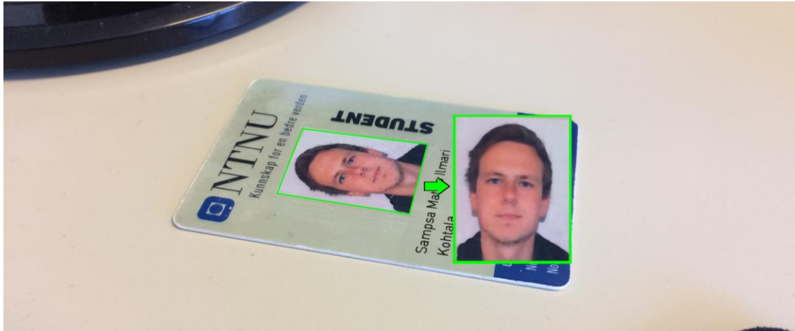
Figure 14: Detect and transform square example with OpenCV. The square is automatically detected and then transformed.
