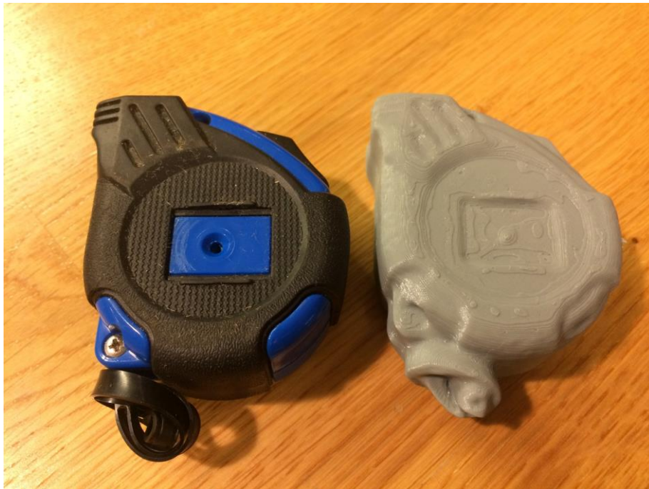
Figure 17: Comparing the real model with a 3D scanned and printed version. The 3D model is scaled, and the background removed manually with CAD before printing.
