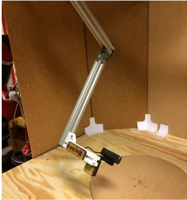
Figure 11: Adjustable camera arm, with buttons for choosing program and adjusting focus.
