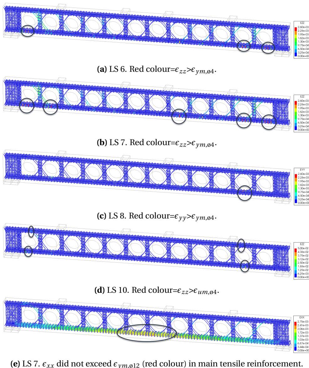
Figure 3.60: RCxcb (3D). Reinforcement strains in x-, y- and z-direction in essential LSs from the NLFEA with the selected solution strategy. Areas of yielding and ultimate strains are marked with circles.
