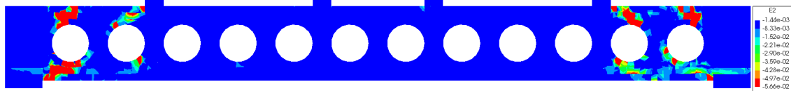
(c) LS 57 (P=284 kN). Red colour= |\epsilon_2| > |\alpha_u| . Blue colour= |\epsilon_2| < |\alpha_c| .
