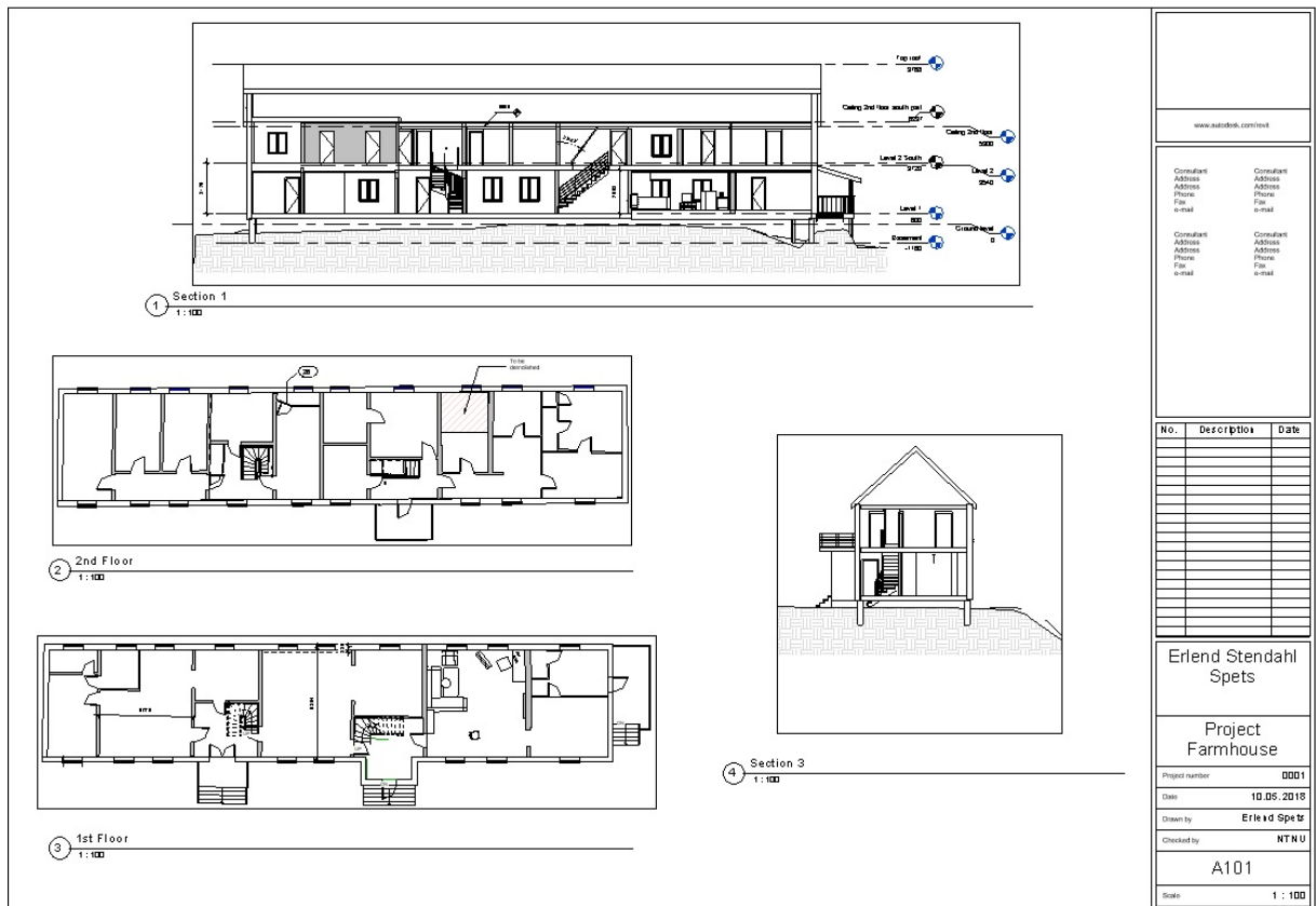
Figure 4.23: An example for how a design drawing sheet for this building could look like. This is including several different views and is easily printed.
