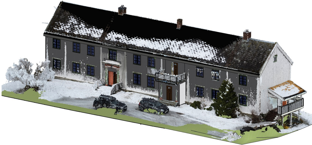
Figure 4.27: BIM and point cloud in the same view: 3D Realistic view from the North-East.
