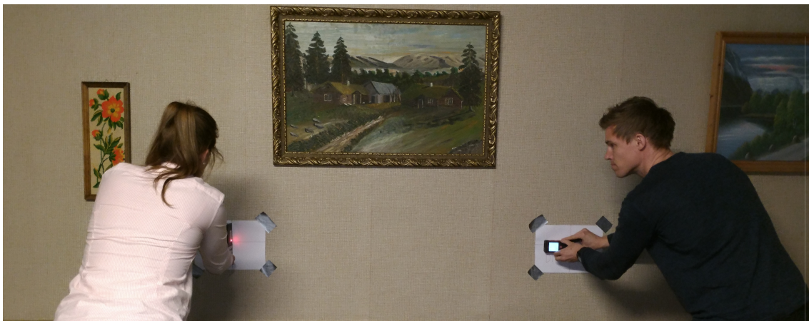
Figure 3.25: The control points placed parallelly on the wall were measured by placing a box on the control point at the right spot.
