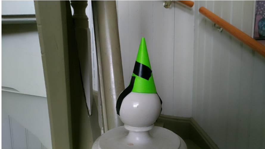
Figure 3.12: Merging points: Coloured cones were placed at central parts of the building during the test.
