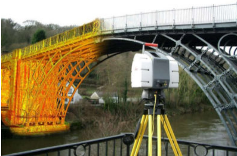
Figure 2.1: Ground fixed LIDAR scanning [1].
