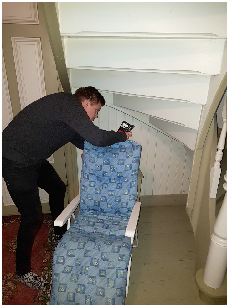
Figure 5.3: By using a phone instead of a laser scanner, it is possible to access more areas of the building from several angles.
