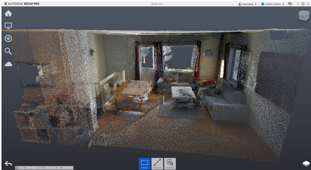
Figure 3.5: Scanned room during daytime with artificial lights on.
