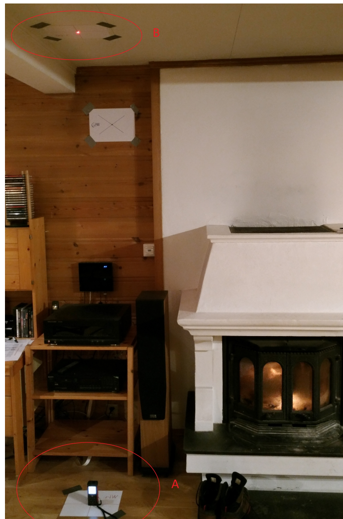
Figure 3.23: Checking that the control point was placed directly opposing the other during experimental setup. The Leica measuring device was placed in control point A, and it was controlled that the laser beam hit the center of control point B
