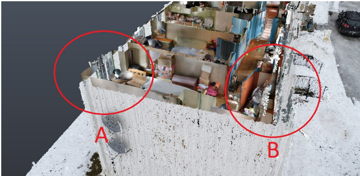
Figure 3.35: Checking error in alignment.
