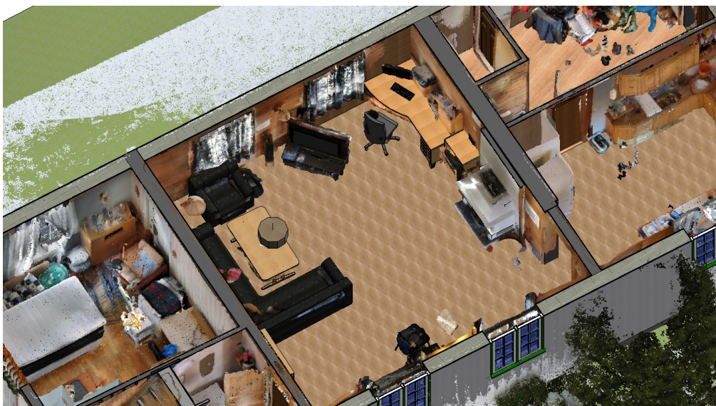
Figure 4.34: A close up 3D Realistic view of the northern livingroom. Most BIM objects fit well with the furniture in the point cloud.
