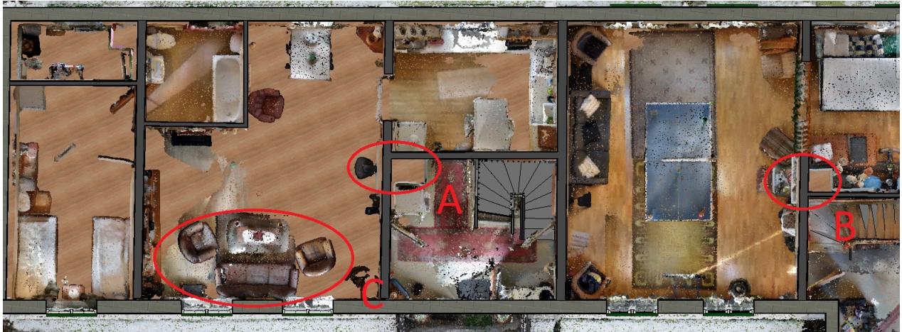
Figure 5.1: Viewing the BIM and the point cloud in the same view. Examples of things that could have been added to the BIM:
