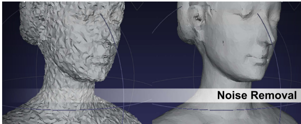
Figure 2.12: An example of MeshLab processing: Smoothing [24].
