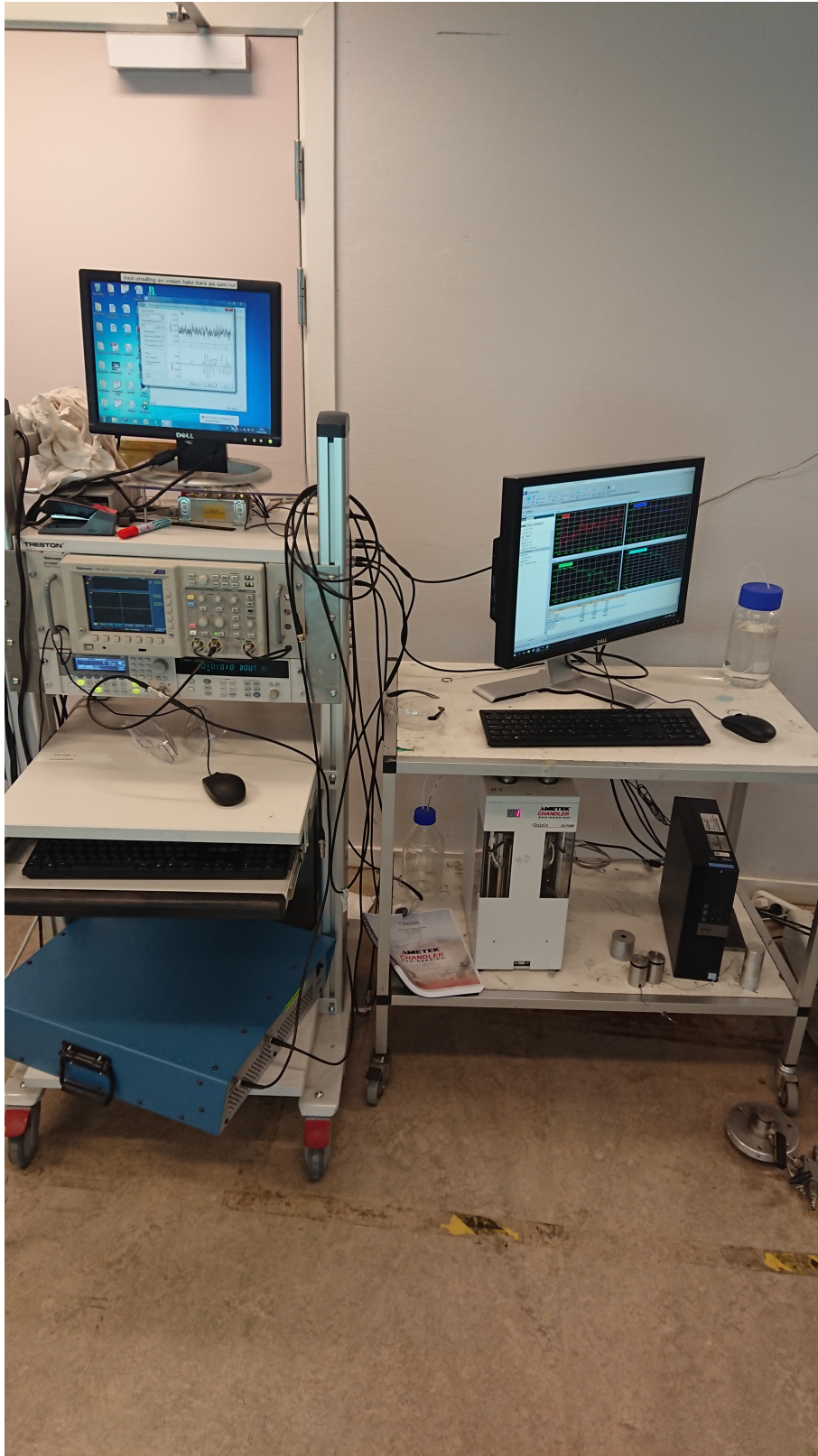
Figure A.4: Computer with data-logging on right and compressional wave velocity measuring on the left
