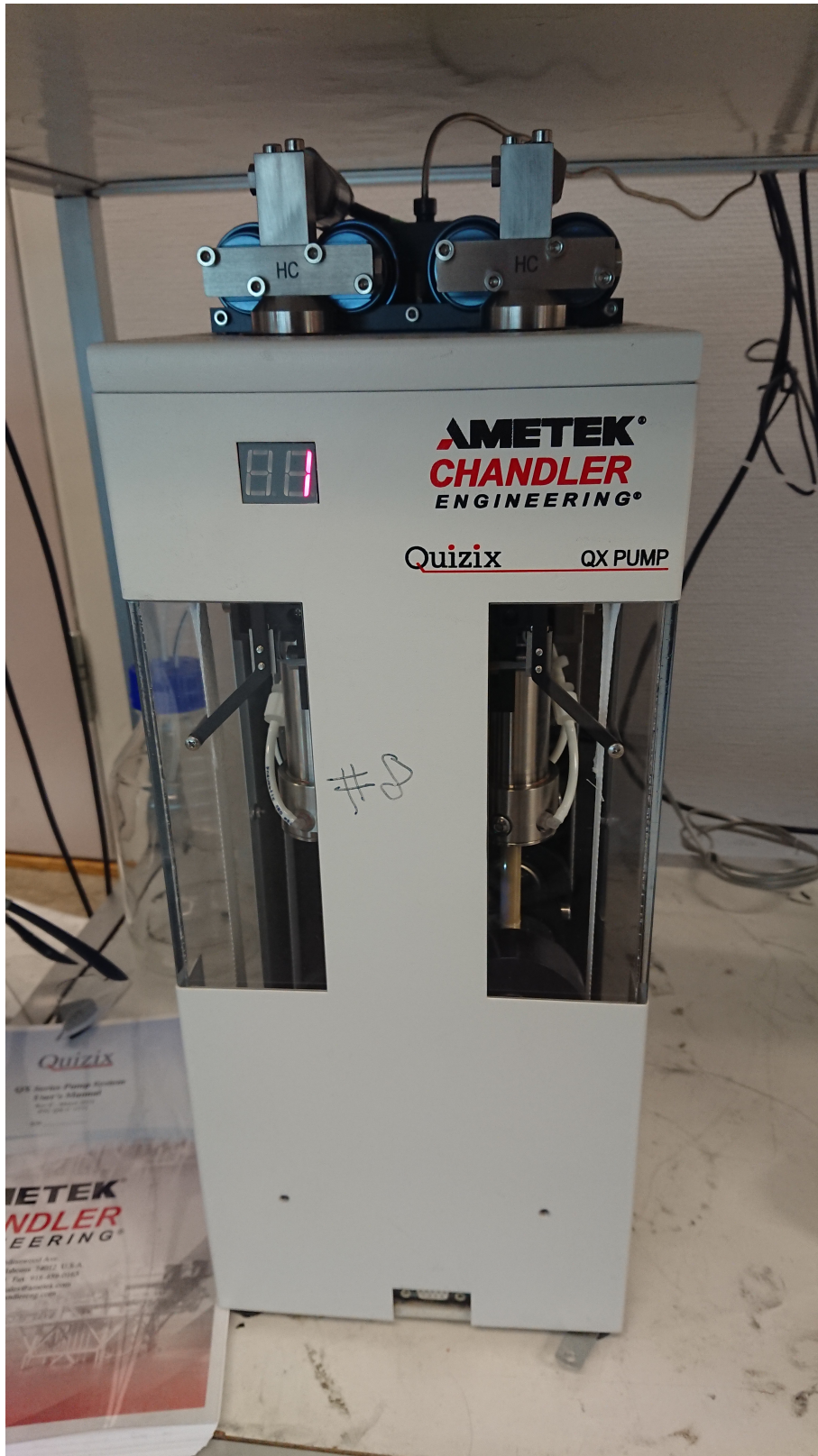
Figure A.3: Pore pressure pump, the two cylinders with a piston each are seen
