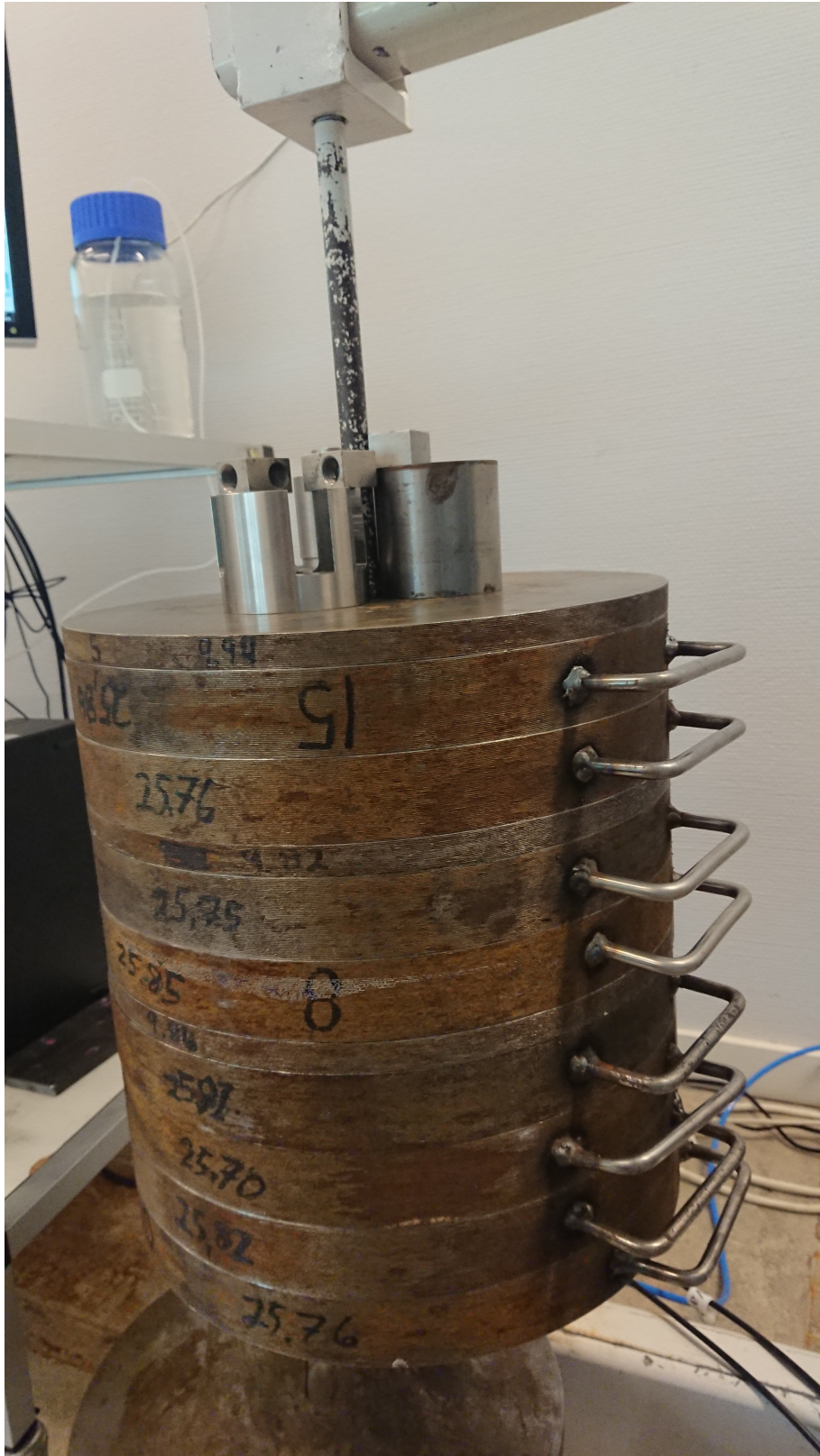
Figure A.5: Deadweight hung off from moment arm
