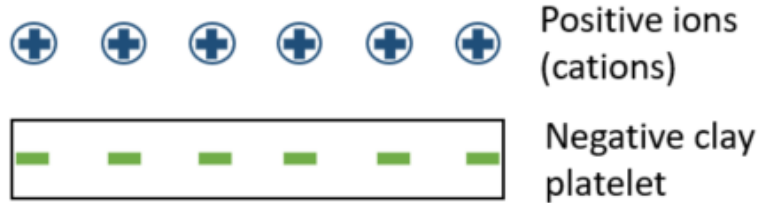
Figure 3.2: Negative clay platelet attracting cations
