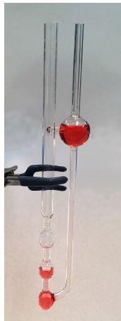
Figure 4.1.1: Cannon-Fenske capillary viscometer filled with oil
