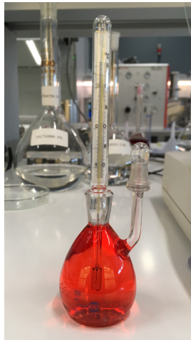
Figure D.0.1: Pycnometer filled with oil
