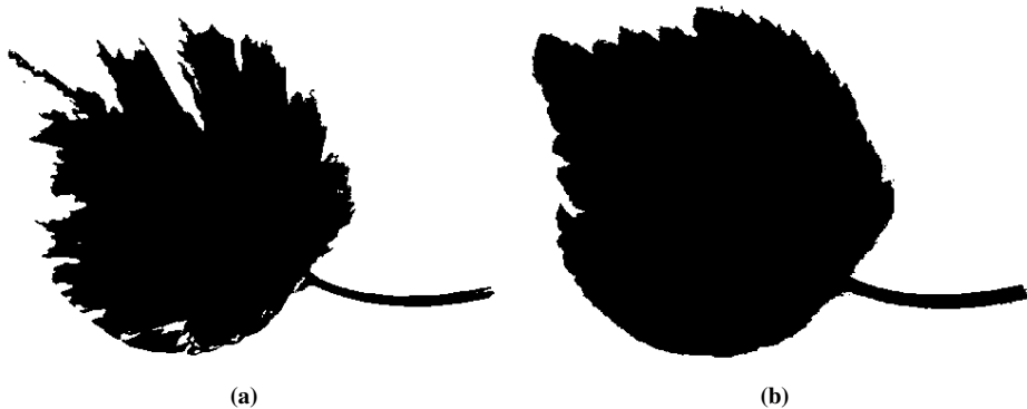
Figure 2.16: Results of segmentation by gray-level thresholding applied on figure 2.15 with intensity thresholds (a) 130 and (b) 228.
