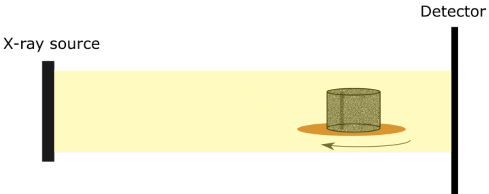
Figure 3.6: Schematic illustration of the setup used for the acquisition of \mu -CT projection images. For each projection image, X-rays propagated from the source towards the HADES rig, which in this figure is represented by the cement cylinder. The detector measured the intensity of X-rays that had been attenuated by the sample. The illustration is based on figure 3.3 in the author's specialization project (Ref. [25]).
