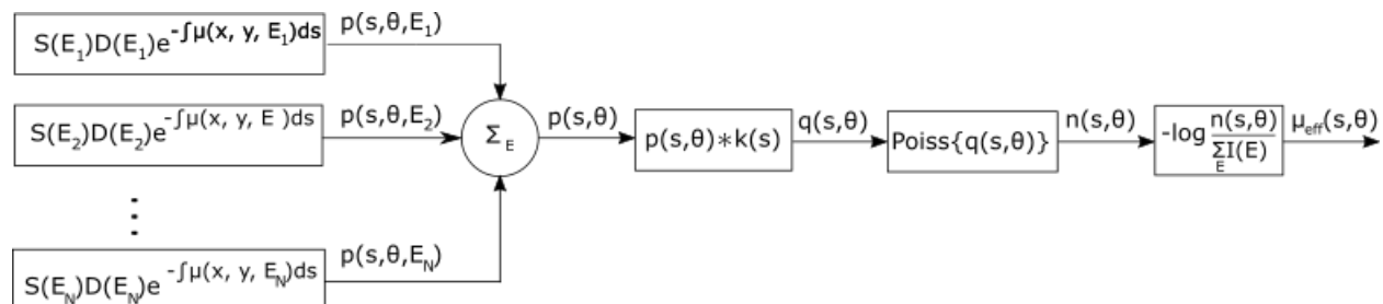
Figure 4.1: The steps in the CT simulations in the form of a cascaded linear system. The first step calculates the projections as a function of energy, giving p(s, \theta, E_i) . The second step summarizes the energy-dependence of the projections into one variable, p(s, \theta) . The third step convolutes the projections with the focal spot distribution and the fourth step applies Poisson noise. The final step calculates the projected effective attenuation coefficients.
