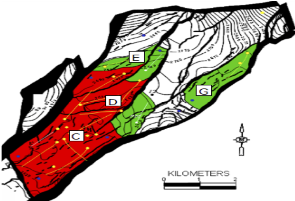
Figure 2.3: Illustration of the shape of the reservoir with the four segments marked. The red area represent the gas cap overlaying the oil, while the green represents oil [2].
