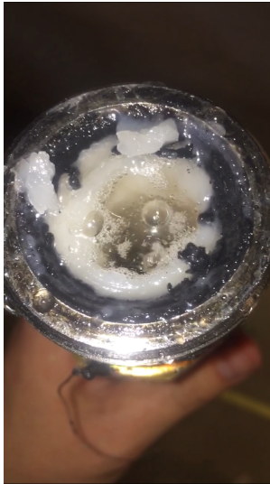
Figure 5.3: Two Gas Bubbles rising out of the pipe section during volume measurements
