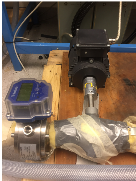
Figure 3.2: Parker Petrol Pump, used to pump waxy oil through the test section
