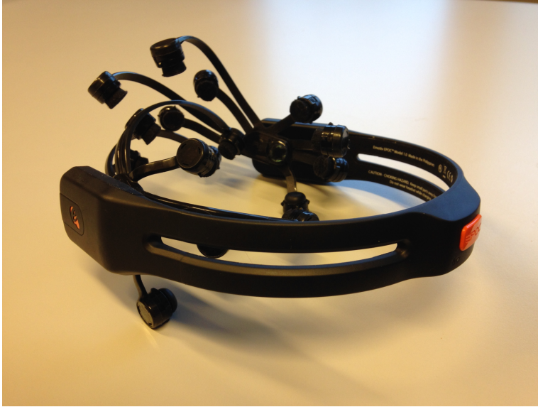
Figure 2.10: The Emotiv EPOC neuroheadset
