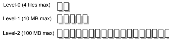
Figure 2.2: Illustration of three levels in LevelDB. Each square is an sstable.
