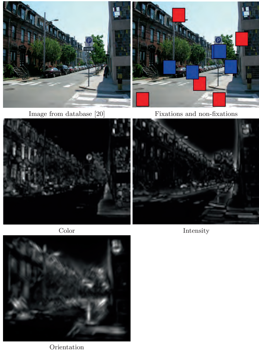
Fig. 1. Figure shows the fixated and the non-fixated regions for an image and the corresponding feature maps obtained by the saliency algorithm [1]. The fixated regions are marked as blue and the non-fixated regions are marked as red
