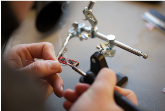
Figure 3.2: Soldering connector pins on 9 DOF sensor
