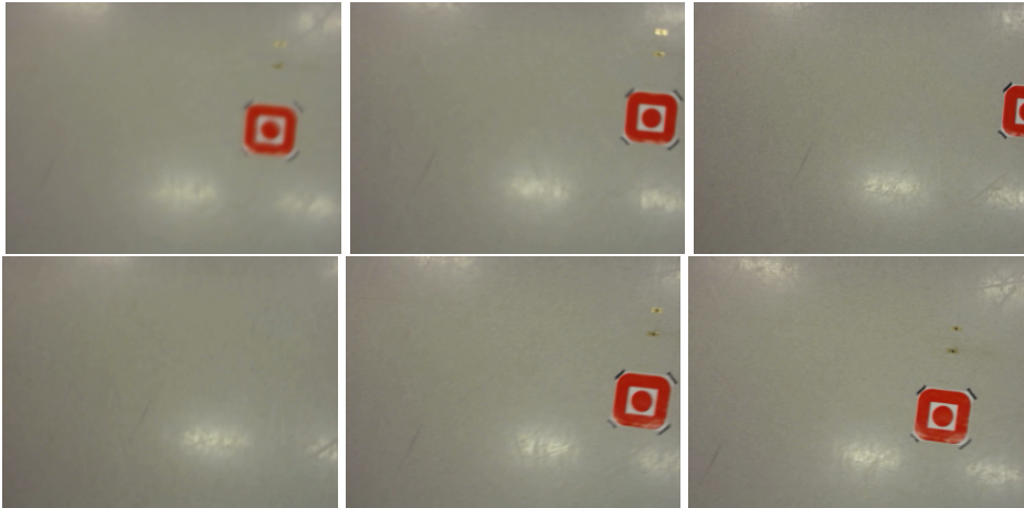
Figure 4.16: The figure shows video images taken from the drones camera. The marker goes out of the cameras field-of-view in picture 3 and 4, and making its recovery in image 5 and 6.
