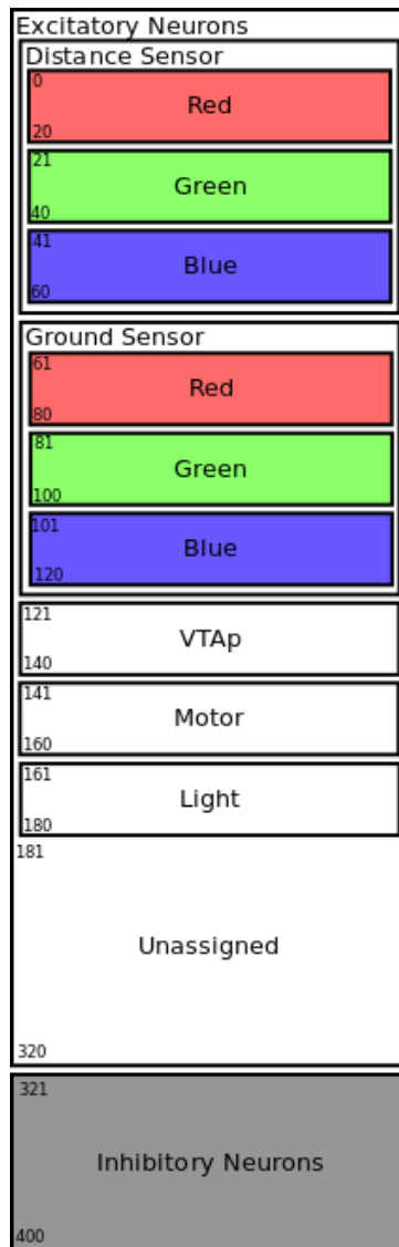
Figure 3.1: Assignment of neurons to various functional areas. Neuron numbers along the left edge. Each neuron group, except the last two, contain 20 neurons.
