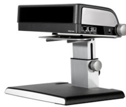
Figure 3.4: The Tobii X60 Eye Tracker.
