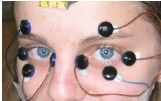
Figure 2.1: By using Electro-oculography (EOG) one could measure the potential differences between eye muscles of the users and thus deduce where the users were looking. (Kumar, 2007)
