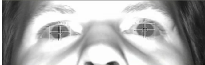
Figure 2.4: Infrared light creates reflexes on the user's cornea that the eye tracker camera can capture and thus find the eyes in the camera image
