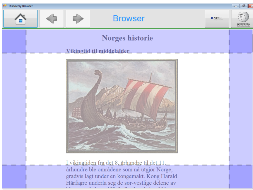
Figure 3.18: The predefined scroll areas for scrolling up, down, sideways and diagonally.
