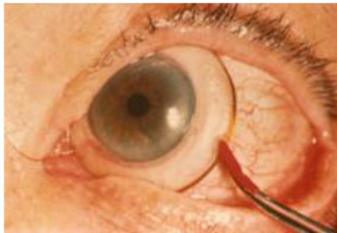
Figure 2.2: A scleral coil contact lens being inserted into a user's eye. When a user kept the head stationary inside a magnetic cage, the user's eye movements created changes in the magnetic field which could be used to measure them. (Kumar, 2007)
