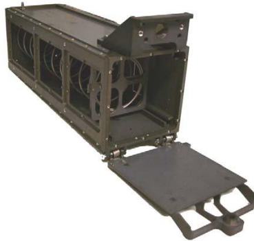
Figure 1.2: The CubeSat P-Pod Mk3. Holds up to 3U CubeSats in place inside the launch vehicle.
