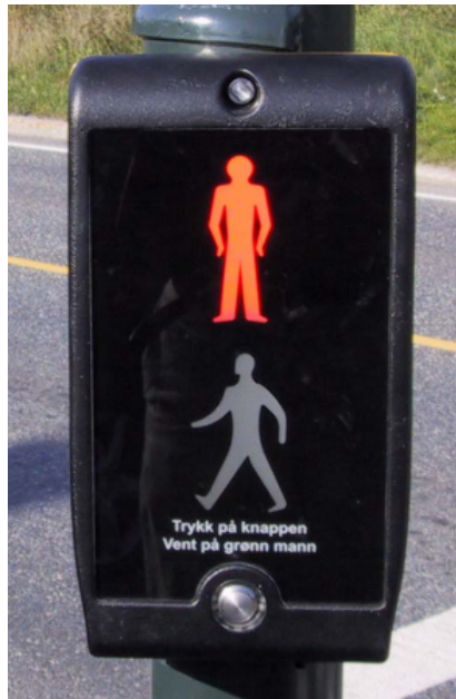
Figure 2.2: Push button with signaling light for pedestrians
