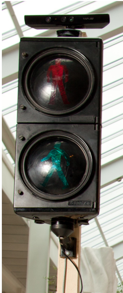
Figure 5.21: The Kinect sensor installed on top of the traffic light
