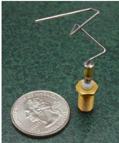
Figure 3.2: ST5-33.142.7 antenna developed through evolutionary design. U.S. NASA. (Public domain)
