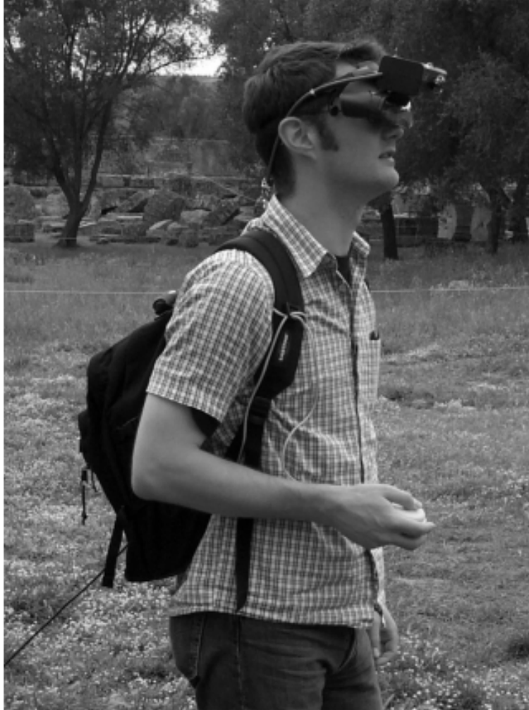
Figure 2.5: The laptop client in the Archeoguide system (photo from Gleue and Dähn [28])
