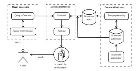
Figure 2.2: Main components of a typical IR system.
