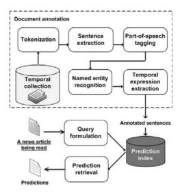
Figure 9.1: Prediction retrieval system architecture.
