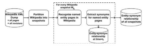
Figure 5.3: System architecture of the module for extracting time-based synonyms.
