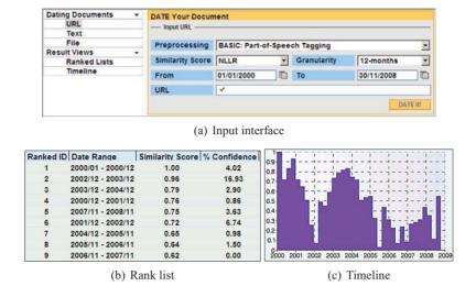
Figure 3.5: Input and output interfaces of the document dating system.
