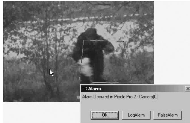
Figure 3.2: An alarm area defined by a four-sided polygon, and a dialog bow appearing when an alarm has been raised.
