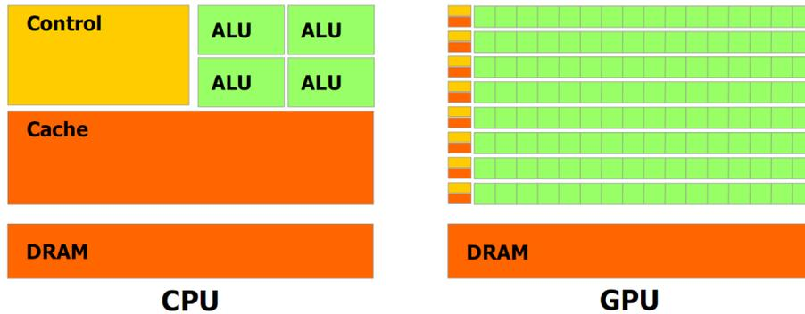
Figure 2.5: The GPU devotes more transistors to processing data, [14].
