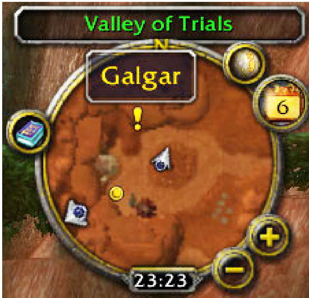
FIGURE 4.10: An implementation of a mini-map with an orthographic top-down view. The map only uses a fraction of the screen space. The player's current location and orientation can be seen together with nearby interesting elements. If the user positions the mouse pointer over those elements, short descriptions about them are displayed in the tooltip. From World of Warcraft by Blizzard Entertainment[20].
