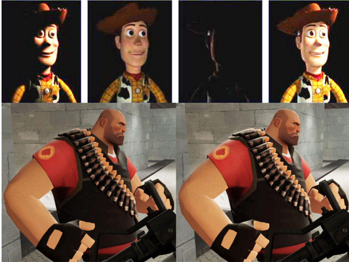
FIGURE 4.3: Top from left to right: Key light, fill light, rim light, all lights. From [64]. Bottom left: Game character without rim lighting. Bottom right: Game character with rim lighting. From [14].
