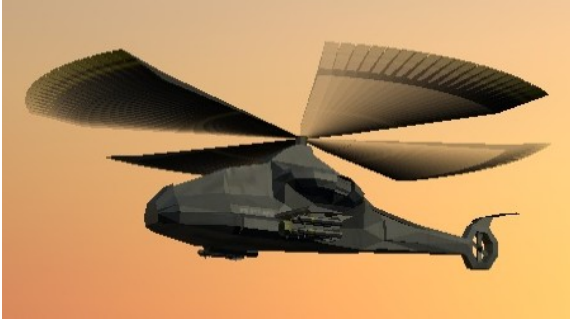
Figure 5.6.: An illusion of motion blur is achieved by rendering gradually more transparent rotor instances.
