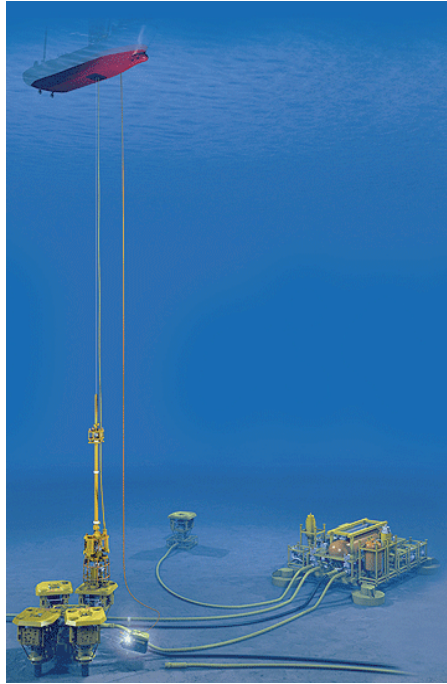
Figure 1 - Illustration of subsea equipment which is remotely maintained by a vessel.
