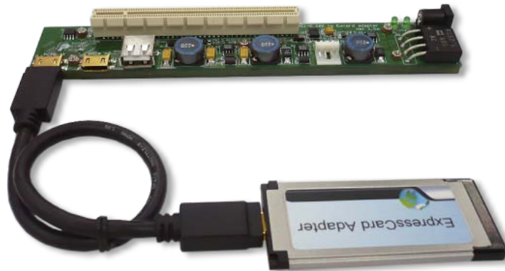
Figure 19: PE4H and E2C2 PCI Express/ExpressCard adapters with HDMI cable
