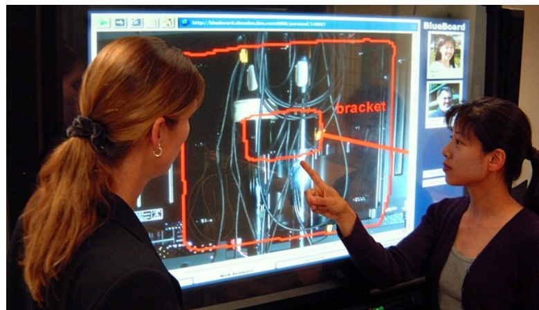
Figure 18: An image showing the BlueBoard in use by two participants. The main part of the screen contains an image that the participants have annotated using the touch screen capabilities. On the left one can see the icons of the two persons who have identified themselves with the display.
