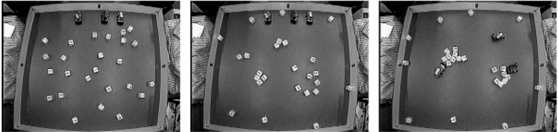
Figure 2.11: Clustering of boxes by DidaBots. Courtesy of the Artificial Intelligence Lab, University of Zurich.
