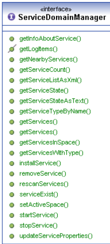
Figure 5.13: Interface for the component ServiceDomainManager .
