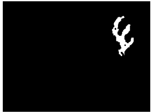
(d) Noise cleaned image. The size of the structuring element was 3 \times 3 , and the minimum region size was 200.
