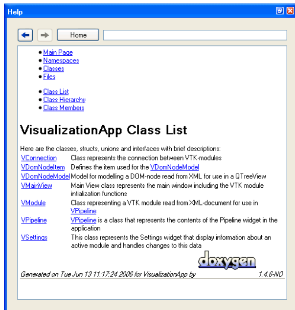
Figure 5.16: The generated HTML project system design class documentation shown in Help Browser.
