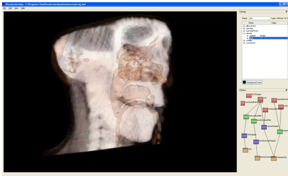
Figure 6.10: The skull is rendered using ray casting while internal cavities and skin are emphasized with an semi-transparent iso-surface.
