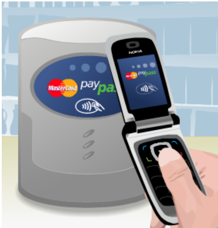
Figure 2.1: An NFC enabled phone tapped to a NFC reader
