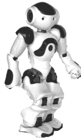
Figure 2.1: Aldebaran Nao TM , the hardware base for the RoboCup Standard Platform League
