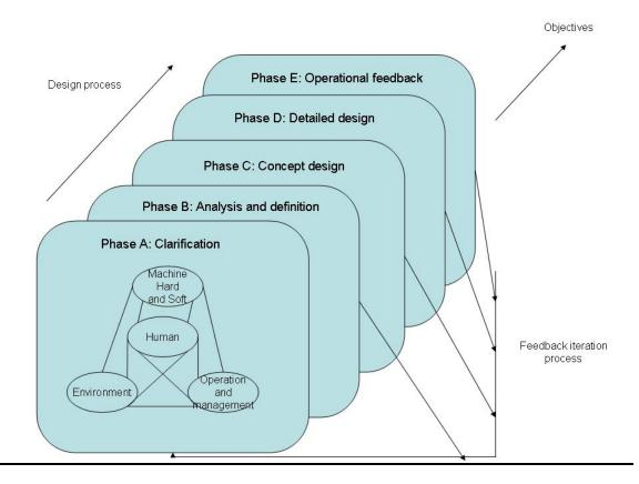
Figure 5-13 Ergonomic approach to system designs from ISO 11064: Ergonomic design of control centers, Part 1: Principles for the design of control centers (2000). [19]
